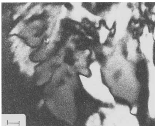
FIGURE 3 Thermotropic inversion wall texture of the soluble polymer obtained by reacting chloroform solutions of bis catechol silane and bis(4- t -butyl-catechol) silane in a 1:1 mole ratio. The specimen was quenched from 180°C. The scale bar represents 5 \mu\text{m} .
